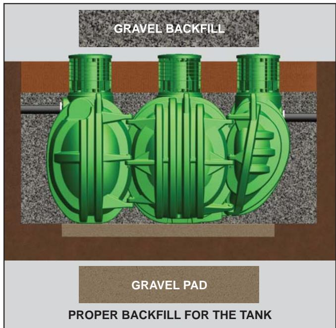
Cover all openings, then begin backfilling with gravel under and around the sloped clarifier. Continue to add gravel until the discharge line from the Singulair Green tank is covered. Proceed to the inlet end of the pretreatment chamber and add gravel until the inlet line is covered. Fine, loose earth may be used to backfill the remainder of the excavation.
