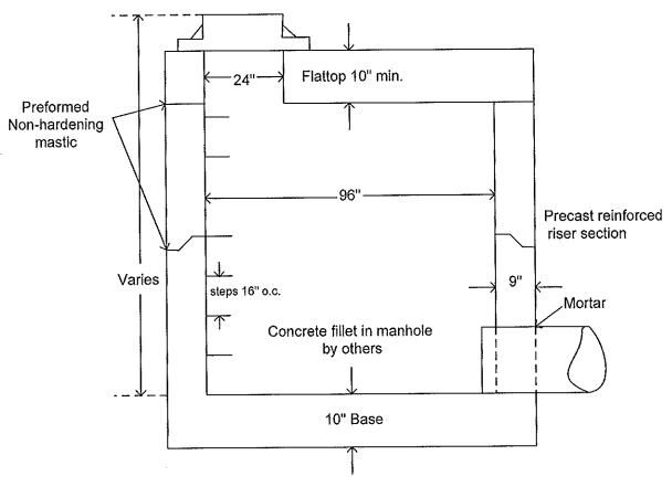
NOTE: ALL MATERIAL SHALL CONFORM TO A.S.T.M. C-478 / A.A.S.H.T.O. M199 AND ILLINOIS STANDARD SPECIFICATIONS.
